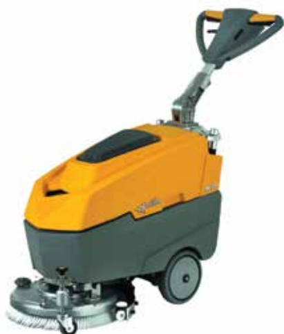
FR 15 E 38 Commercial Walk Behind Scrubber Drier - AC Power Cleaning Width: 385mm / Squeegee Width: 450mm Performance (Theoretical): 1540m 2 /hr Cleaning Solution Tank: 15ltrs / Recovery Tank: 17ltrs
